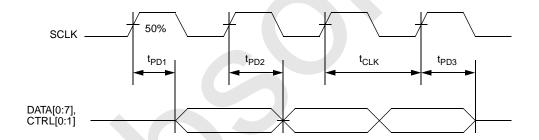
Figure 4-1. SCLK to Data Valid Timing Waveform
