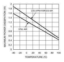
Figure 48. Maximum Power Dissipation
