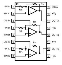
Figure 1. 16-Pin SSOP - Top View  $R_F = R_G = 327\Omega$
