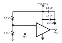
Figure 40. Recommended Single Supply Inverting Gain Circuit, Gain = −1 V/V
