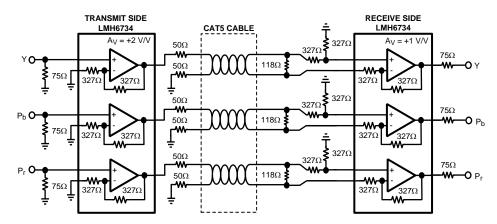
Figure 45. Component Video Transmission Over UTP (CAT5)
