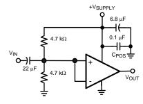
Figure 43. Alternate Unity Gain Compensation
