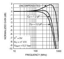
Figure 42. Frequency Response for Circuit in Figure 41
